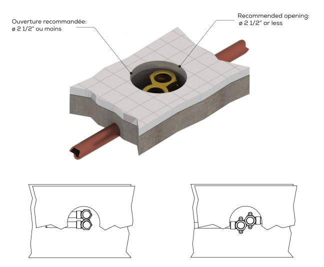
Optimize your rough configuration for a minimum C-C between hot & cold inlets (see examples). The orientation of the pair of supply connections is independent from the final spout position.
